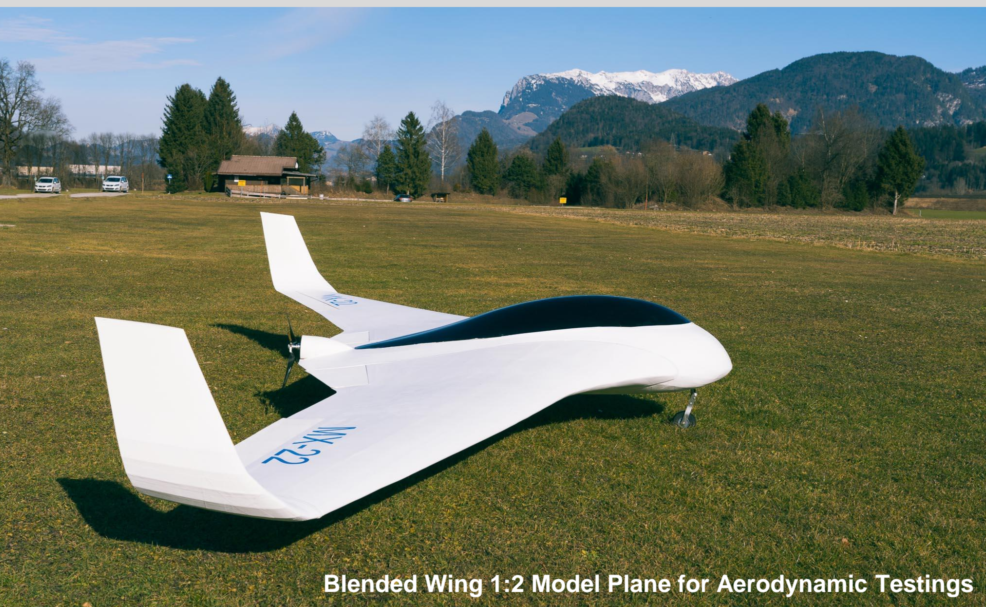
Blended Wing 1:2 Model Plane for Aerodynamic Testings
